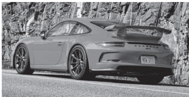
At the GT3's core is a 3.8-litre, 475-horsepower, non-turbo, flat-six engine. JUSTIN PRITCHARD
